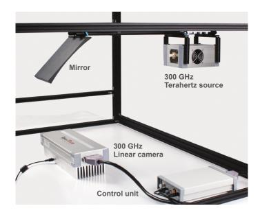
The camera has both internal and external synchronization features. The internal synchronization can operate with an externally modulated source to reduce the noise and improve image quality.
