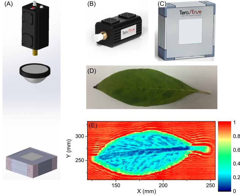
**Fig 1** (A) Schematic illustration of the experimental setup. The radiation beam produced by the IMPATT-diode source is collimated by a PTFE lens with a focal distance of 50 mm. The power distribution within the beam is probed with the imaging camera. (B) and (C) Photos of the camera and the IMPATT source. (D) and (E) A regular, visible light photo and a sub-THz image of a tree leaf. Image colors indicate the transmission coefficient values.
